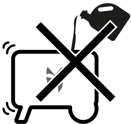
Remember to switch off the engine before refuelling.
